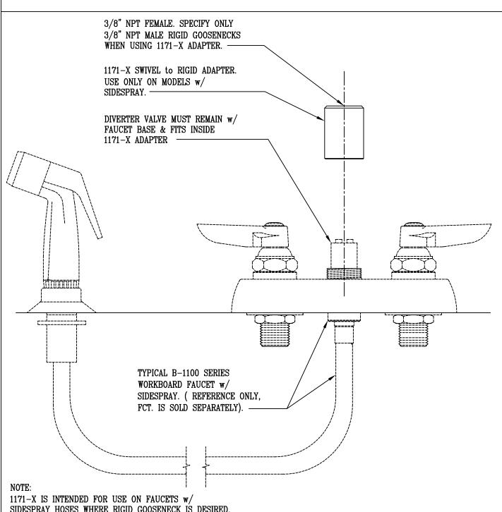
1171-X IS INTENDED FOR USE ON FAUCETS w/SIDESPRAY HOSES WHERE RIGID GOOSENECK IS DESIRED. B-413 SWIVEL to RIGID ADAPTER WILL NOT FUNCTION WHERE SIDESPRAY HOSE IS PRESENT.
