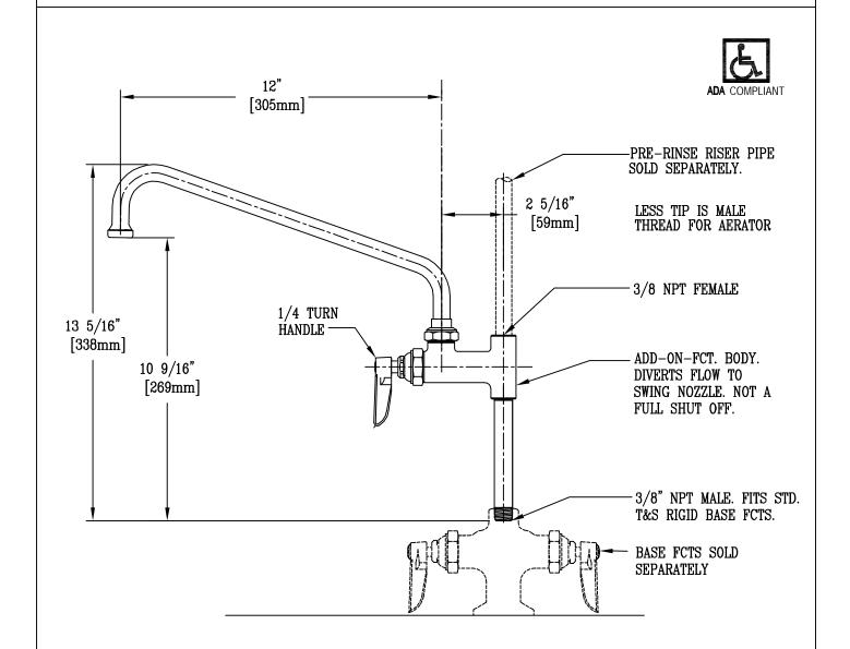
NOTES: 1. THE ADD-ON FAUCET IS AN ADDITION TO PRE-RINSE UNITS AND IS INSTALLED IN OUTLETS OF BASE MIXING FAUCETS OF UNITS BEFORE FITTING RISER PIPE, AS SHOWN.
