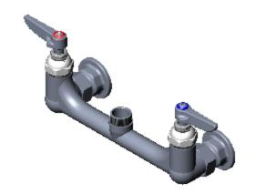
Swivel Outlet Accepts Standard Swing Nozzles such as 062X Lever Handles w/ Colored Indexes Ø2" [51mm] w/ 1/2" NPT 8" [203mm] Female Inlets Adjustable from 7 3/4" to 8 1/4" [197mm to 210mm]
