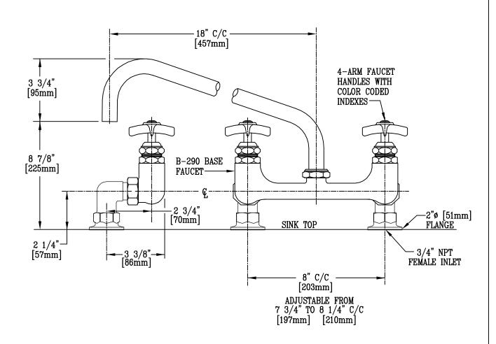
NOTE: DRILL 1 1/4"ø [32mm] HOLES ON 8"C/C IN SINK TOP.
