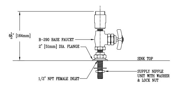
NOTE: DRILL 1 1/4" [32mm] HOLE ON 8"C/C IN SINK TOP.
