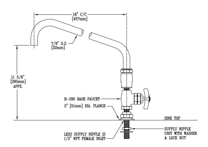
NOTE: DRILL 1 1/4" [32mm] HOLE ON 8"C/C IN SINK TOP.
