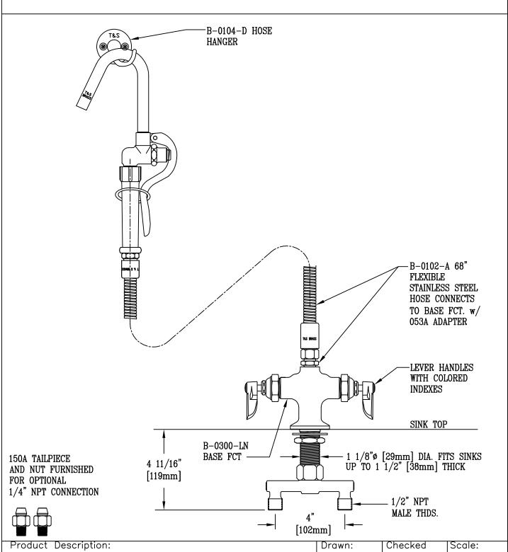
Single Hole Deck Mount Mixing Faucet w/ B-0102-A Hose & Hook Nozzle
