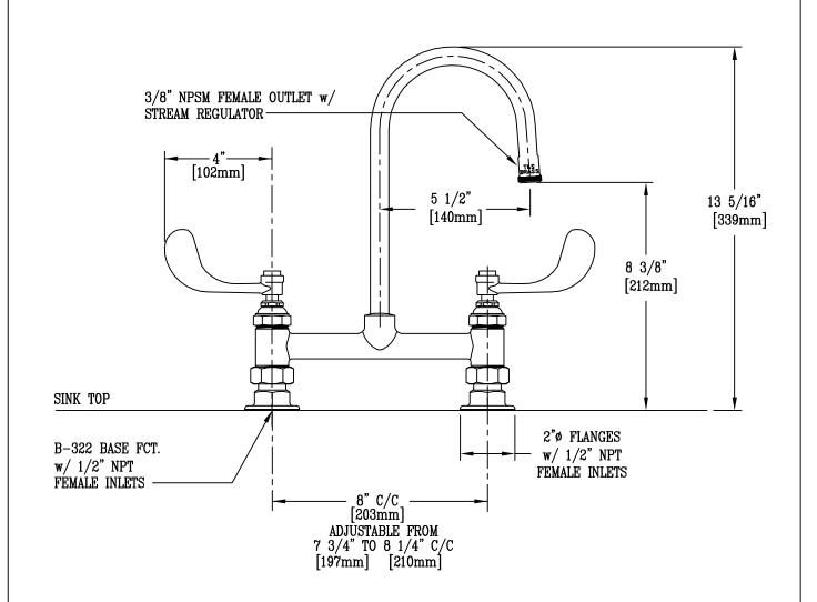
8" c/c DECK MOUNTED SURGICAL SINK FCT. w/ 120X RIGID GOOSENECK, STREAM REGULATOR, BWH4" HANDLES, & 1/2" NPT FEMALE INLETS
