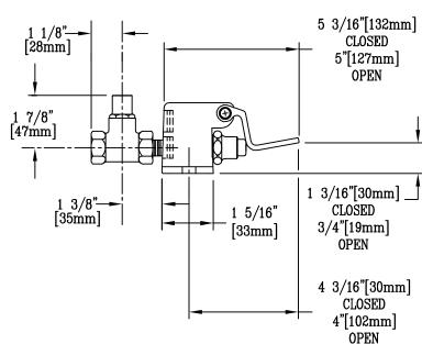
NOTE 1. INLETS & OUTLET ARE 1/2" NPT FEMALE NOTE 2. FURNISHED WITH (2) WOOD MOUNTING SCREWS
