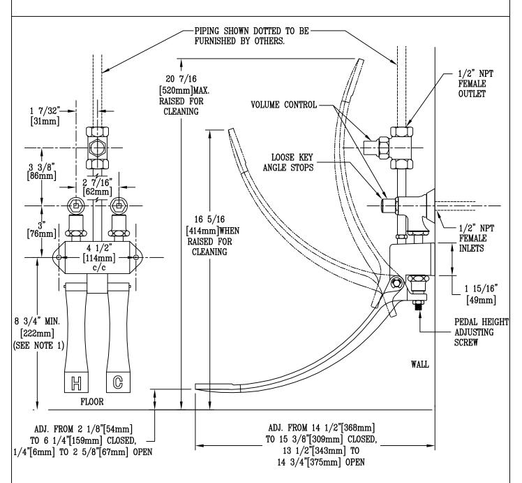
NOTE 1. ALL PEDAL POSITION DIMENSIONS ARE BASED ON A RECOMMENDED MIN. MTG. HEIGHT OF 8 3/4"[222mm] ABOVE FIN. FLOOR
