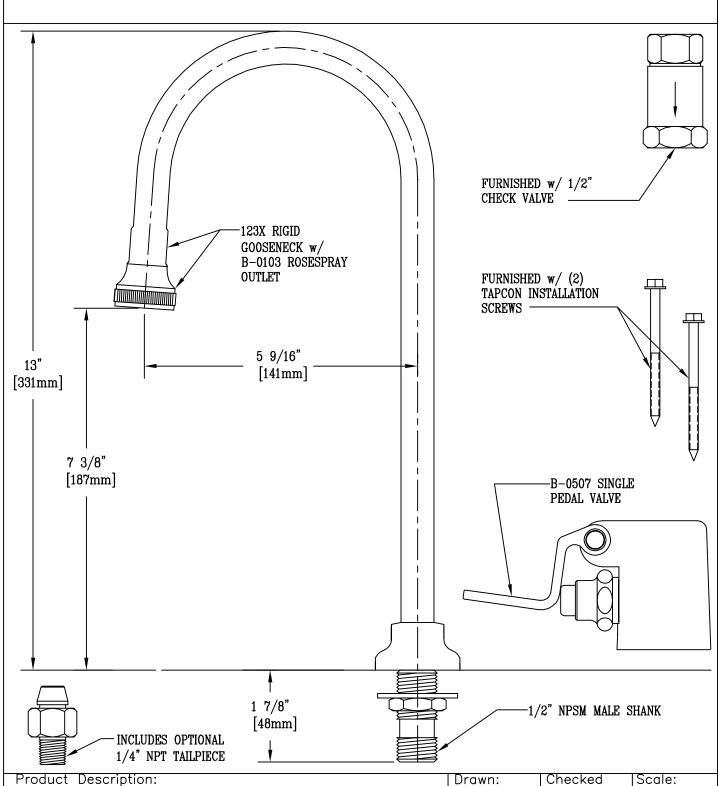
SINGLE PEDAL VALVE, CHECK VALVE, TAPCON INSTALLATION SCREWS,
