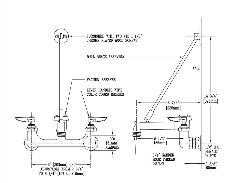
CARTRIDGES INCLUDE SPRING CHECKS TO PREVENT CROSSFLOW OF HOT & COLD WATER
