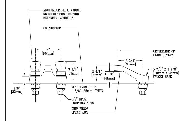
FLOW ADJUSTABLE FROM INSTANTANEOUS SHUTOFF TO EXTENDED FLOW BY EXTERNAL ADJUSTMENT.
