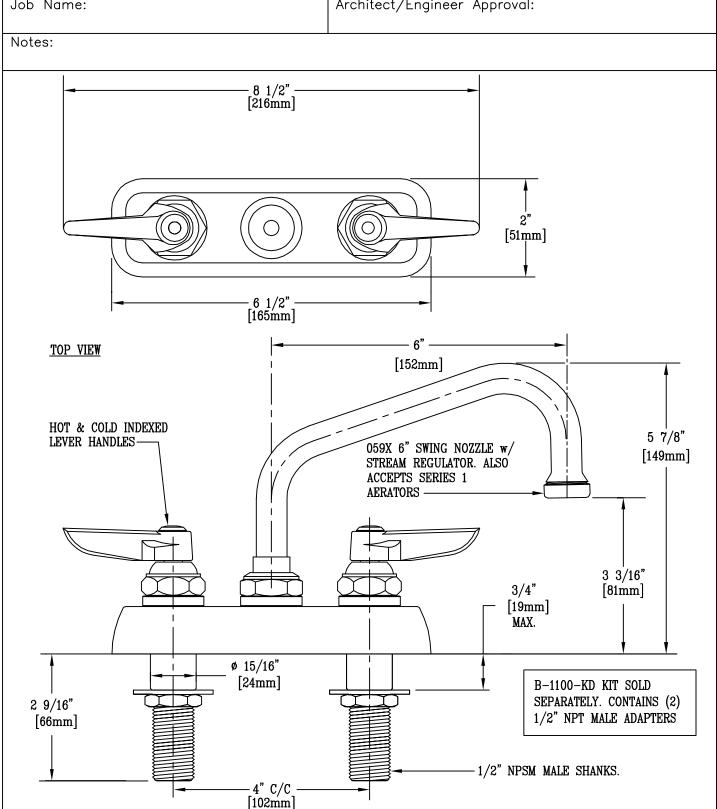
Product Description: WORKBOARD FAUCET w/ 1/2" NPSM MALE EXTENDED SHANKS, 4" INLET CENTERS, 059X 6" SWING NOZZLE, STREAM REGULATOR, LEVER HANDLES
