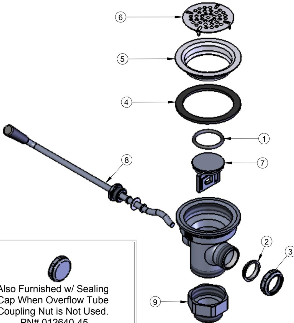
Also Furnished w/ Sealing Cap When Overflow Tube Coupling Nut is Not Used.
