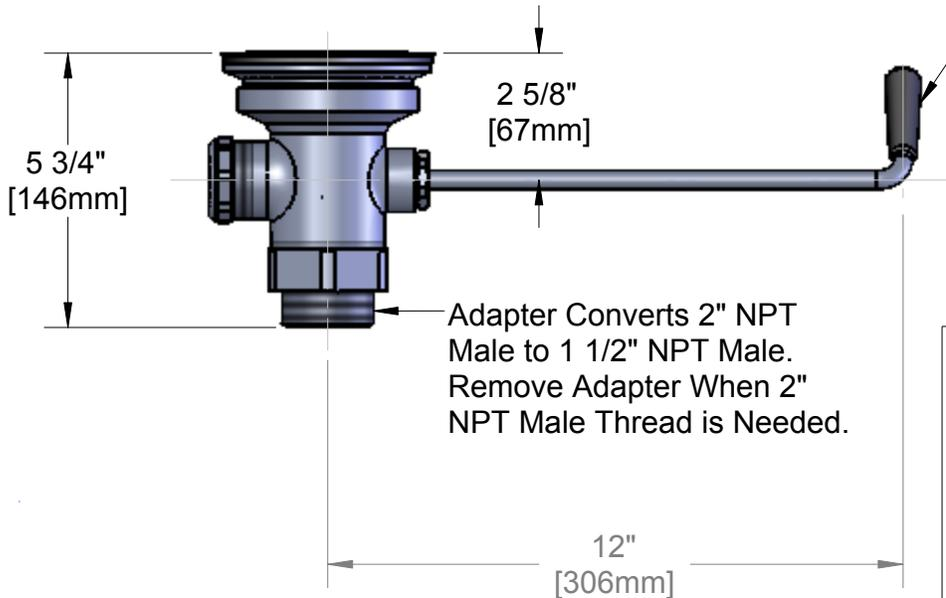
Adapter Converts 2" NPT Male to 1 1/2" NPT Male. Remove Adapter When 2" NPT Male Thread is Needed.
