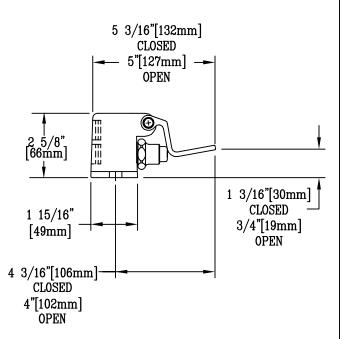
NOTE 1. INLETS & OUTLET ARE 1/2" NPT FEMALE NOTE 2. FURNISHED WITH (2) WOOD MOUNTING SCREWS
