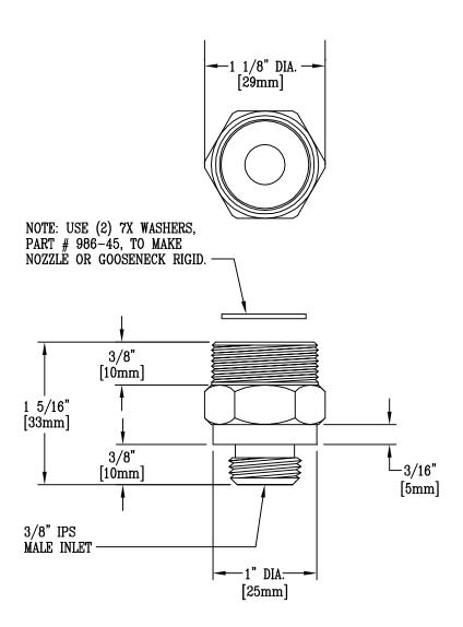
THIS ADAPTER PIECE FITS INTO MANY T&S FAUCETS WITH TEFLON TAPE OR CEMENT TO CONVERT A RIGID OUTLET TO A SWIVEL OUTLET. (ALSO FITS T&S SWING NOZZLES AND GOOSENECKS).
