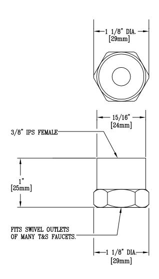
THIS ADAPTER PIECE FITS INTO MANY T&S FAUCETS WITH CEMENT TO CONVERT A SWIVEL OUTLET TO A RIGID OUTLET.
