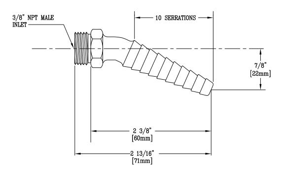
NOTE: BL-5550-26 SERRATED TIP IS USED ON SIDE OUTLETS OF TURRETS, OUTLETS, OR PANEL FLANGES, AND IN OTHER APPLICATIONS IN WHICH A SMALL HEX SHOULDER IS NECESSARY TO AVOID INTERFERENCE OR CONTRIBUTE TO APPEARANCE.
