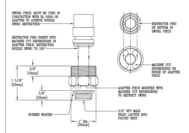
SWING GOOSENECK OR SPOUT MUST BE MODIFIED WITH ADAPTER PIECE, AND SWIVEL PIECE AS SHOWN. SWIVEL PIECE IS FITTED WITH RESTRICTOR PINS WHICH INSERT INTO SMALL, MACHINE CUT DEPRESSIONS IN BOTTOM OF ADAPTER PIECE, AND THUS RESTRICT SWING OF SWIVEL PIECE (AND NOZZLE) TO A 100 DEGREE SWING.
