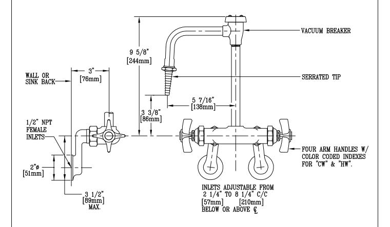
NOTE: INLET ARMS ALSO AVAILABLE WITH H-H INTEGRAL LOOSE KEY STOPS. SEE MODEL NO. BL-5580. WHEN H-H STOPS ARE USED, INLETS ARE THEN ADJUSTABLE FROM 2 1/4" TO 6" [57mm to 152mm].
