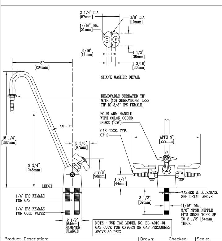
COMBINATION GAS & WATER FIXTURE WITH (2) GAS COCKS, GOOSENECK WITH SERRATED TIP, 3/8" IPS INLETS, & 8" GOOSENECK SPREAD.
