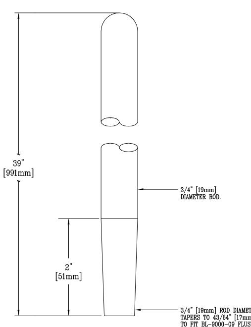
3/4" [19mm] ROD DIAMETER TAPERS TO 43/64" [17mm] DIA. TO FIT BL-9000-09 FLUSH PLATE.
